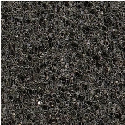
Sonitech is an open cell polyether foam with excellent sound absorption properties. The material has good mechanical strength, is very flexible, durable and flame retardant.
