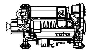
FUEL SUPPLY: 8 mm FUEL RETURN: 8 mm EXHAUST 50 mm (M4.56 = 60 mm) SEAWATER INTAKE 20 mm
