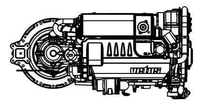
FUEL SUPPLY: 8 mm FUEL RETURN: 8 mm EXHAUST 50 mm (M4.56 = 60 mm) SEAWATER INTAKE 20 mm
