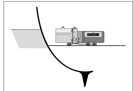
The filler cap for the balance pipe\* should always be on top, at the highest point.
