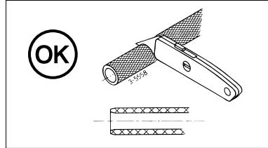
Never cut the hose with a saw (sawdust in the hydraulic system will create problems) or by clipping (this deforms the hose).
