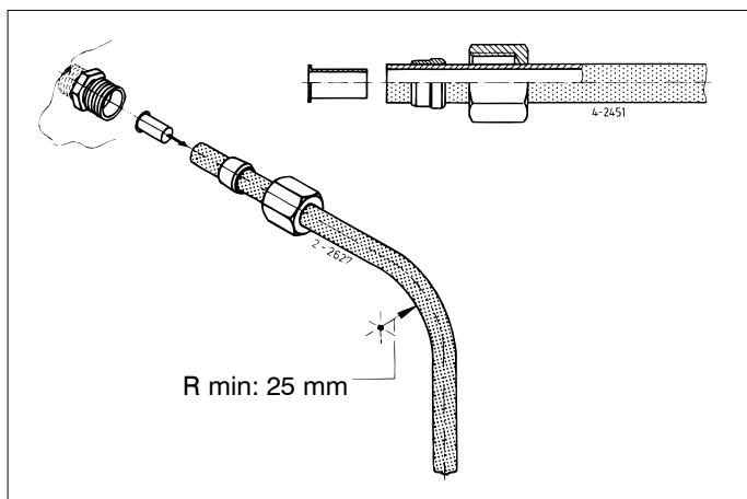
After cutting the nylon tube, fit the coupling nut and olive on the tube and fit the support sleeve inside the tube.
