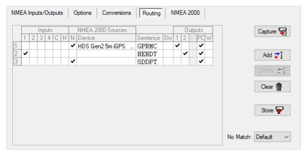
Figure 53: Routing table on an NMEA 2000 enabled MiniPlex-3
