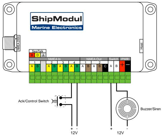
Figure 62: AIS MOB Alarm connections
