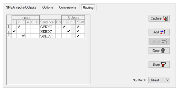
Figure 52: Routing table on an NMEA 0183-only MiniPlex-3
