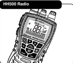
Refer to the foldout at the front of this manual to identify the various controls and indicators on your radio. Throughout this manual you will be instructed to “Press” or to “Press and Hold” various buttons (except “Push to Talk”) on the radio. “Press” means a momentary press of approximately one (1) second. “Press and Hold” means to hold the button down for approximately two (2) seconds.
