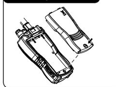
When your rechargeable batteries begin to discharge too quickly, it is time to install a new battery pack. Your radio will also operate with five (5) high-quality AA alkaline batteries, using the included alkaline battery tray.
